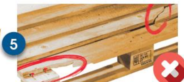
More than 2 broken deck boards
