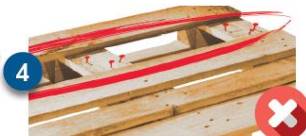
Missing deck board
