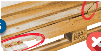
More than 2 broken deck boards
